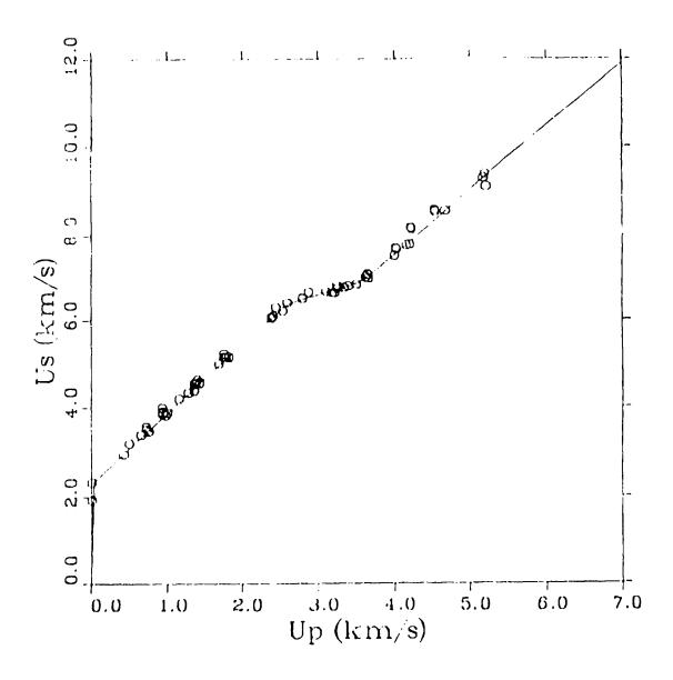
Figure 1 - The calculated principal Hugoniot for polycarbonate (volid line) is compared to the experimental data of Ref. 2.
